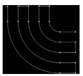
COORDINATE TRANSFORMATION CYCLES EXAMPLE: USING THE THREE MIRROR IMAGE COMMANDS
